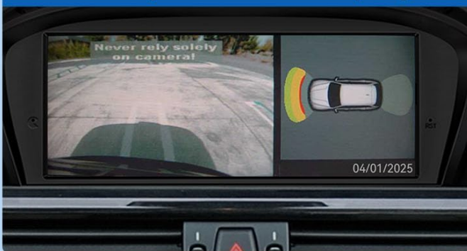
Figure 2.5: Illustration of how the XTRONS unit retains essential original car functions, including iDrive system control, amplifier system, original radio, CD, Bluetooth, backup camera display, and steering wheel controls.
