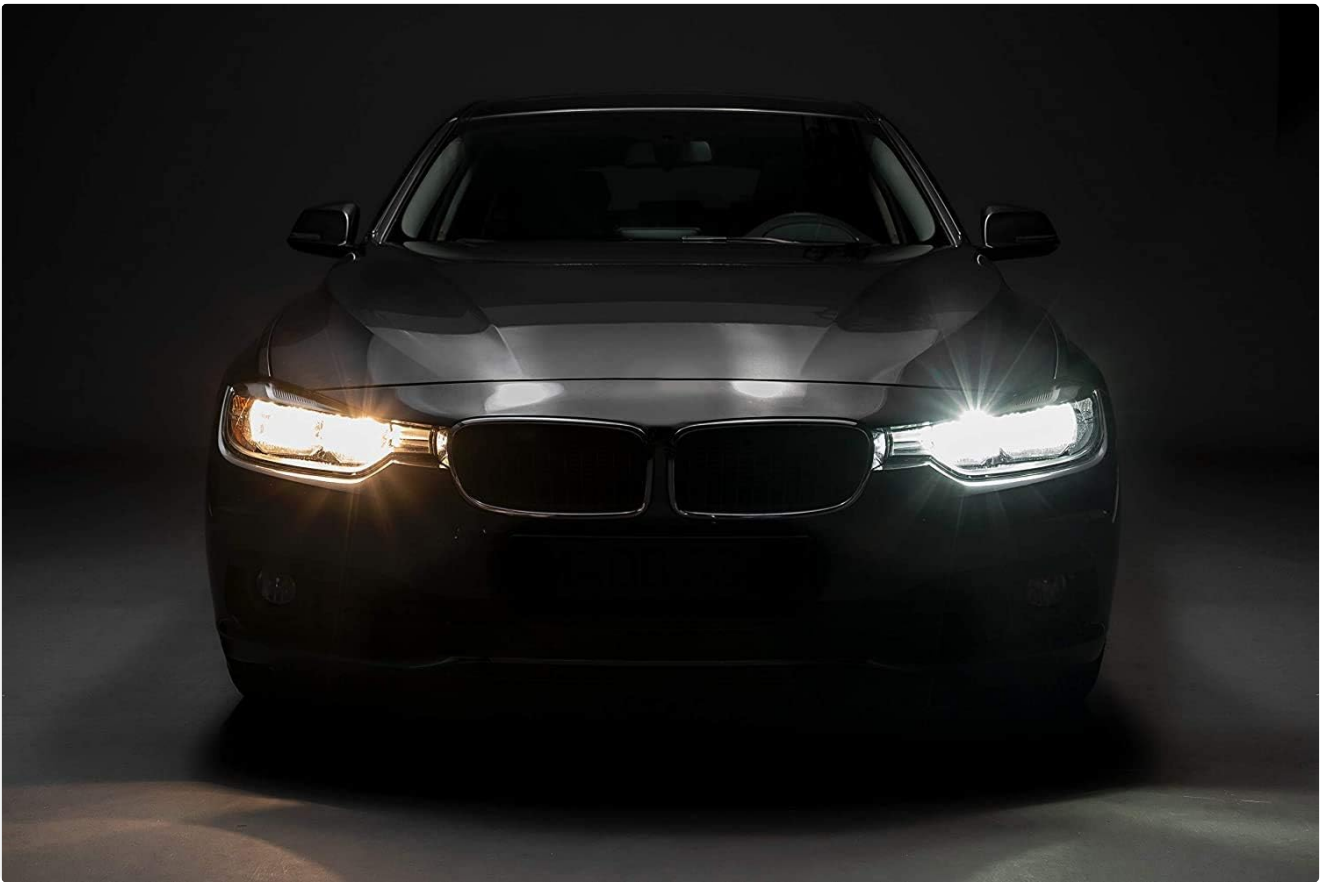
Image: A car demonstrating the difference between a standard halogen headlight (left) and an OSRAM LED headlight (right), highlighting the brighter, whiter light output of the LED.
