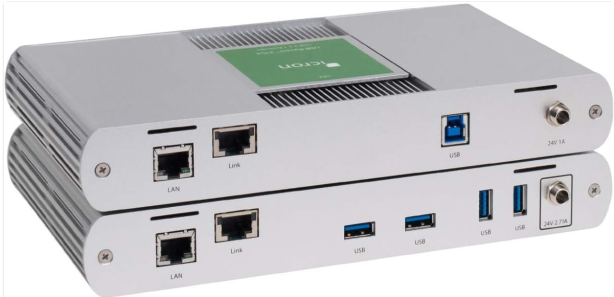
Figure 1: The Icron ICR-3104 Raven USB 3-2-1 Extender System. This image displays two units stacked, showcasing their various ports. The top unit (Local Extender or LEX) has a LAN port, a Link port, a USB 3.1 Type-B port for host connection, and a 24V 1A power input. The bottom unit (Remote Extender or REX) features a LAN port, a Link port, multiple USB 3.1 Type-A ports for connecting peripheral devices, and a 24V 2.71A power input. Both units are silver-colored with heat dissipation fins on the sides.
