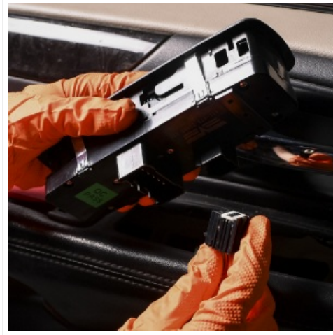
Image 4.1: Using a trim tool to carefully pry the old switch assembly from its housing in the door panel.
