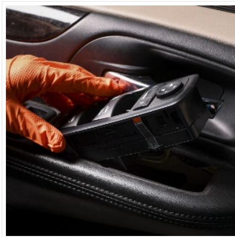
Image 4.2: Detaching the wiring harnesses from the rear of the switch module.
