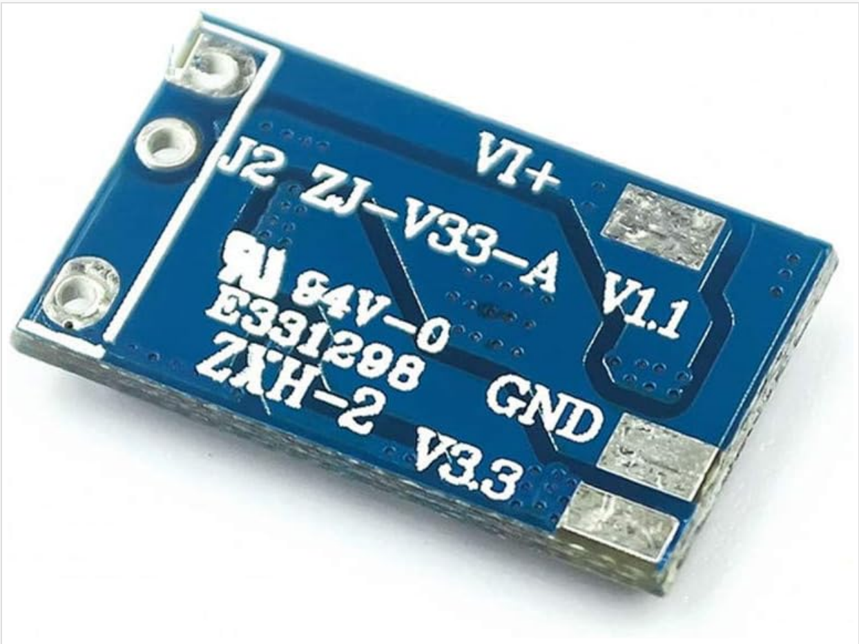
Figure 1: Module Bottom View with Pinout. This image displays the underside of the MP2307DN module, clearly labeling the input voltage (V1+), ground (GND), and 3.3V output (V3.3) pins for connection.
