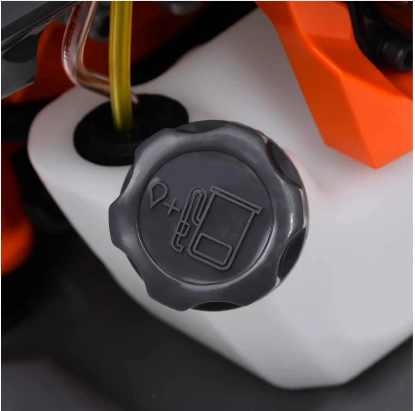
Figure 4: Fuel cap indicating petrol and oil mixture.
