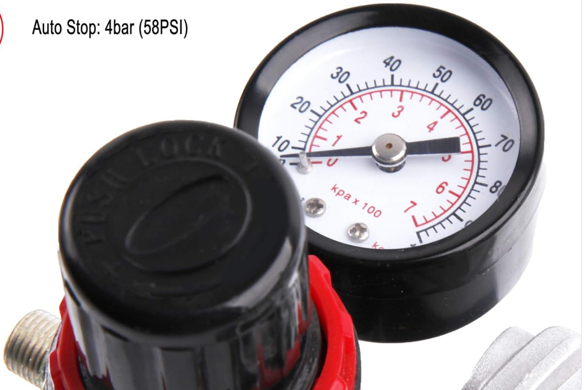
Figure 3.1: Compressor gauge illustrating the auto-start and auto-stop pressure settings.
