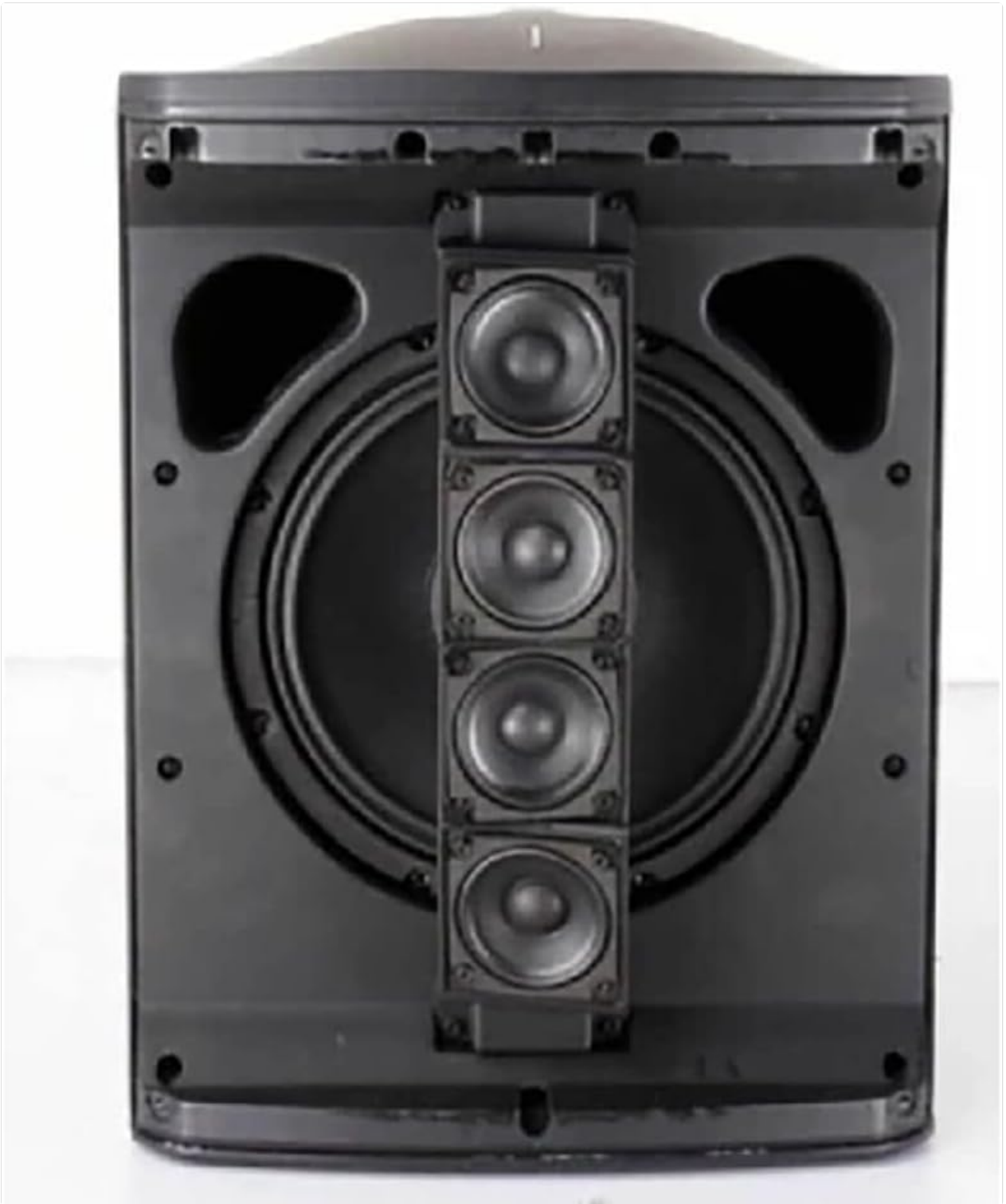
Figure 3.3: Front view of the EPT1 PA System with the grille removed, revealing the 10-inch woofer and the vertical line array speakers.
