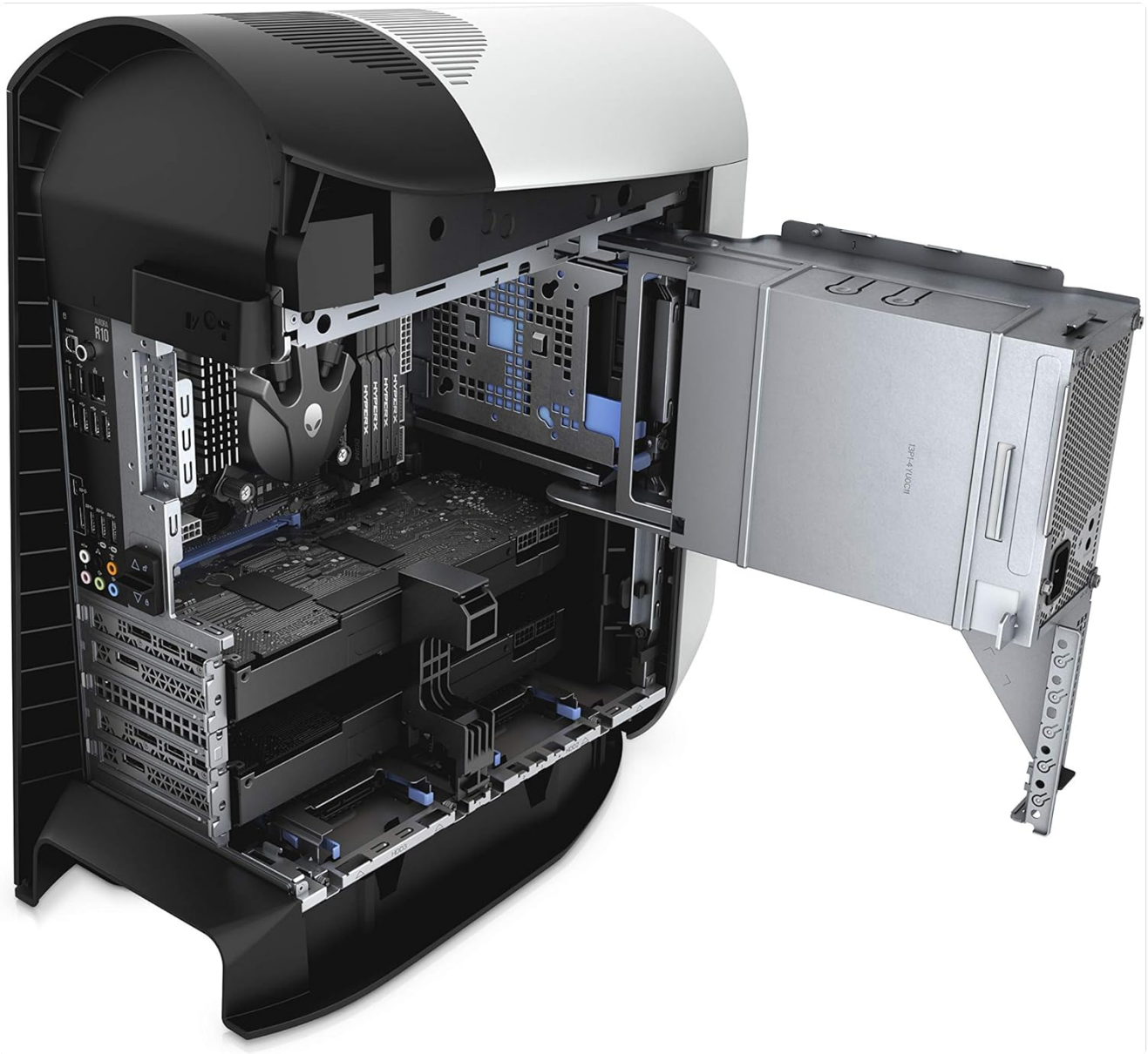
Figure 4.1: Internal view of the Alienware Aurora R10, showing the arrangement of key components such as the CPU, RAM, and graphics card.
