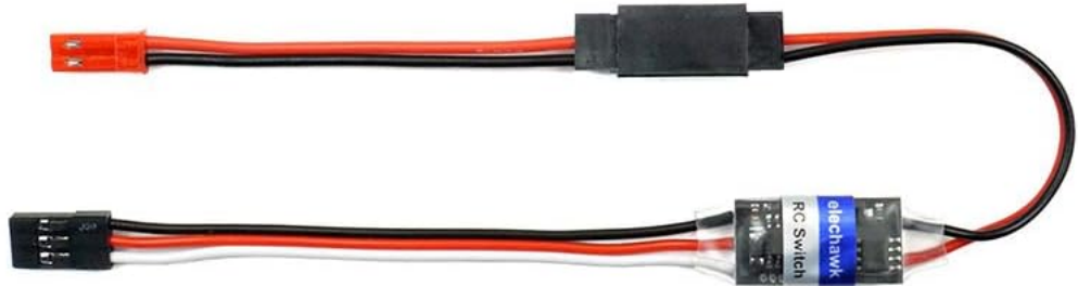
Figure 5.3: This image illustrates the output port compatibility of the RC switch, showing how it can be connected using either Futaba/JR or JST type connectors.
