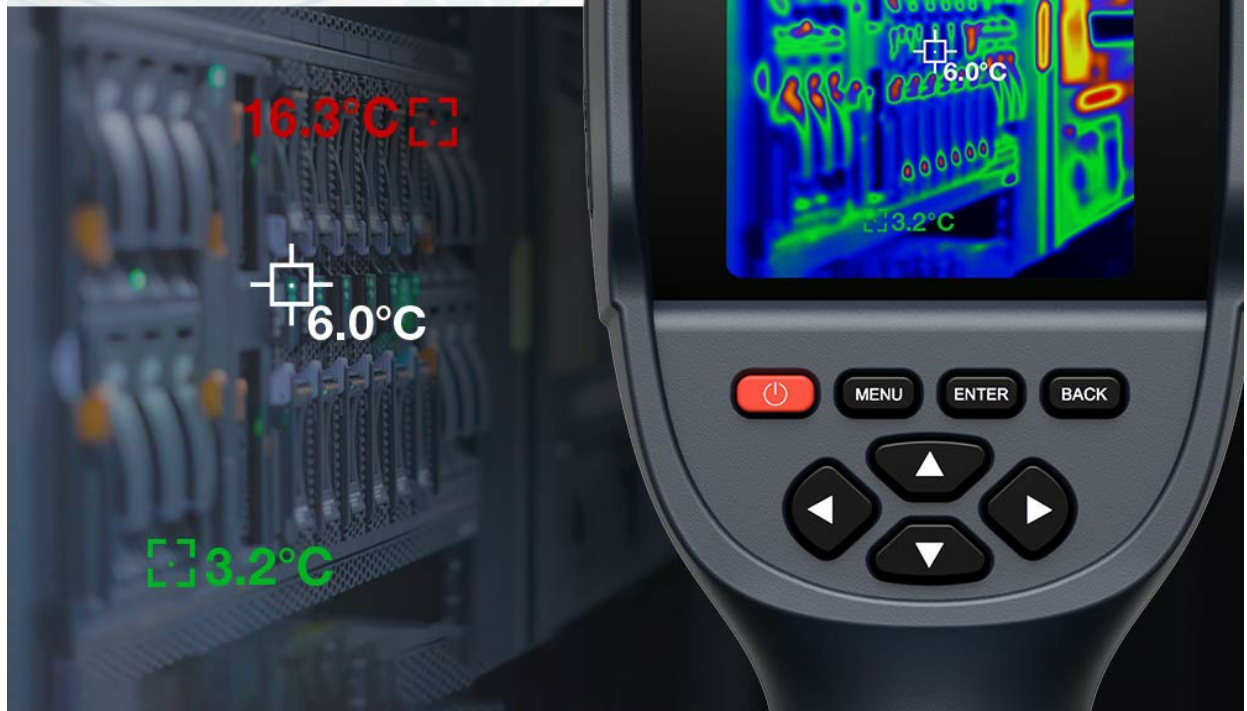
Figure 4.3: Screen displaying the automatic cold and hot spot tracker, highlighting temperature extremes within the image.
