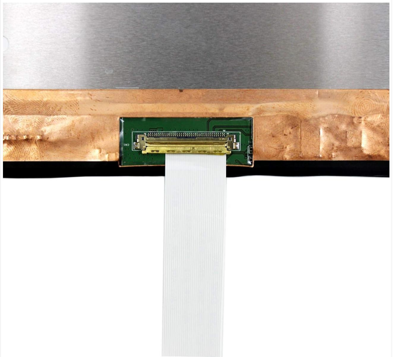
Figure 5.2: Connecting Signal Cable to LCD Screen.
