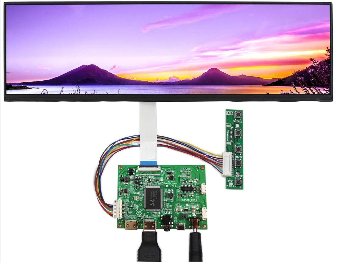
Figure 5.1: Assembled LCD Screen and Controller.
