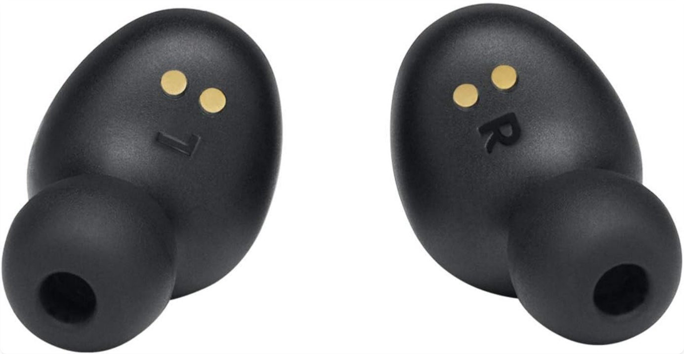
Image: The underside of the JBL Tune 115TWS earbuds, displaying the metallic charging contacts that connect with the charging case.
