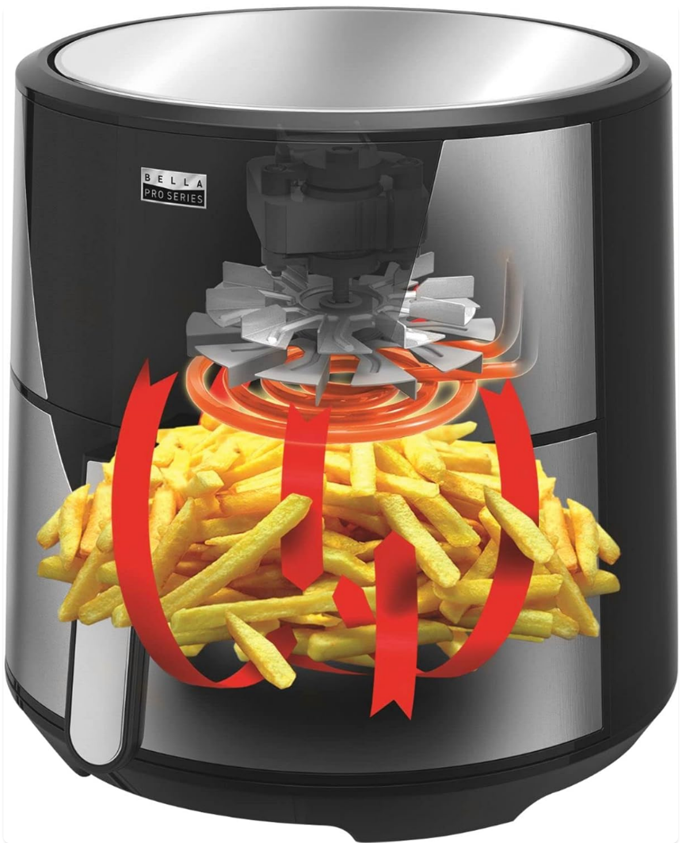
Figure 2: Internal view illustrating the High Performance Circular Heat Technology, showing hot air circulating around food for even cooking.
