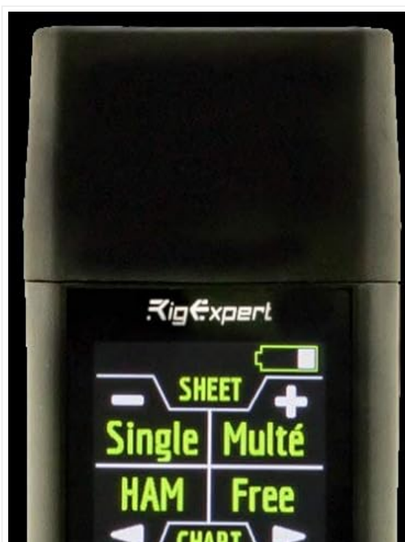
Figure 2.2: Close-up view of the RigExpert Stick Pro Antenna Analyzer, showing the display and control buttons, with the attached lanyard.
