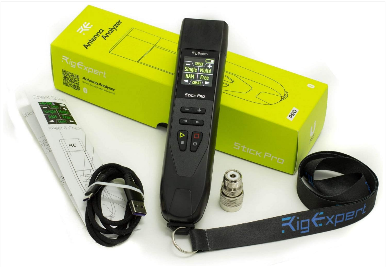
Figure 2.1: RigExpert Stick Pro Antenna Analyzer with its original packaging, USB cable, and lanyard. The device features a color display and control buttons.
