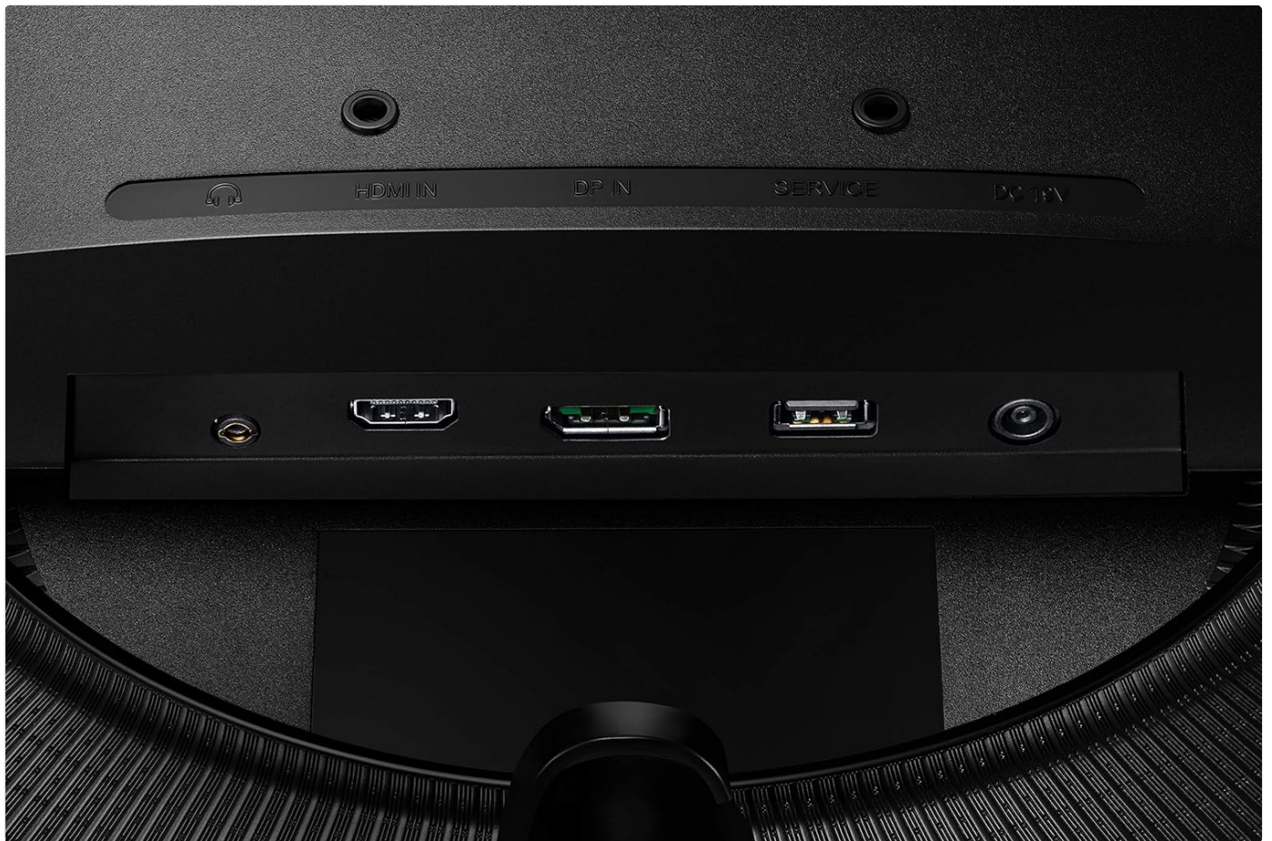
Image: Detailed view of the monitor's rear input panel, showing HDMI, DisplayPort, and power connections.
