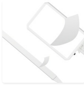
Image: Illustration of peeling the adhesive backing from the LED strip.
