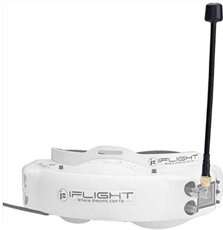
Figure 2.2: Antenna Connected to FPV Goggles. The antenna should be securely attached to the video receiver (VRX) port on your goggles for clear video reception.
