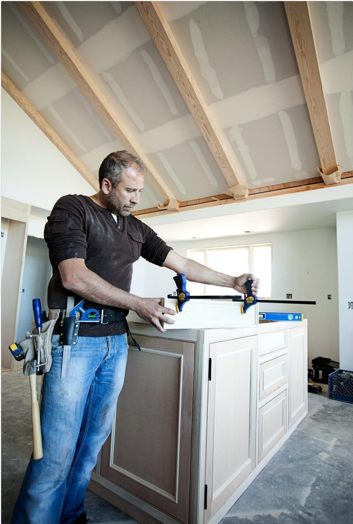
Image: A person demonstrating the use of an IRWIN QUICK-GRIP clamp to hold a workpiece.
