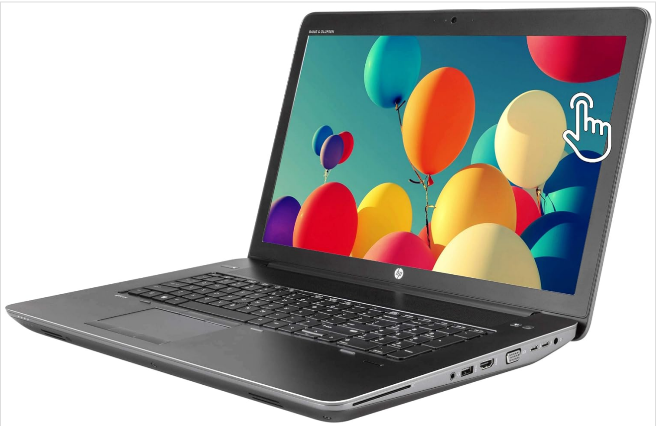
Right-side view of the HP ZBook 17 G3 laptop, showing the various ports including USB, HDMI, VGA, and a Thunderbolt 3 (USB-C) port. The screen is open, displaying the same vibrant wallpaper.
