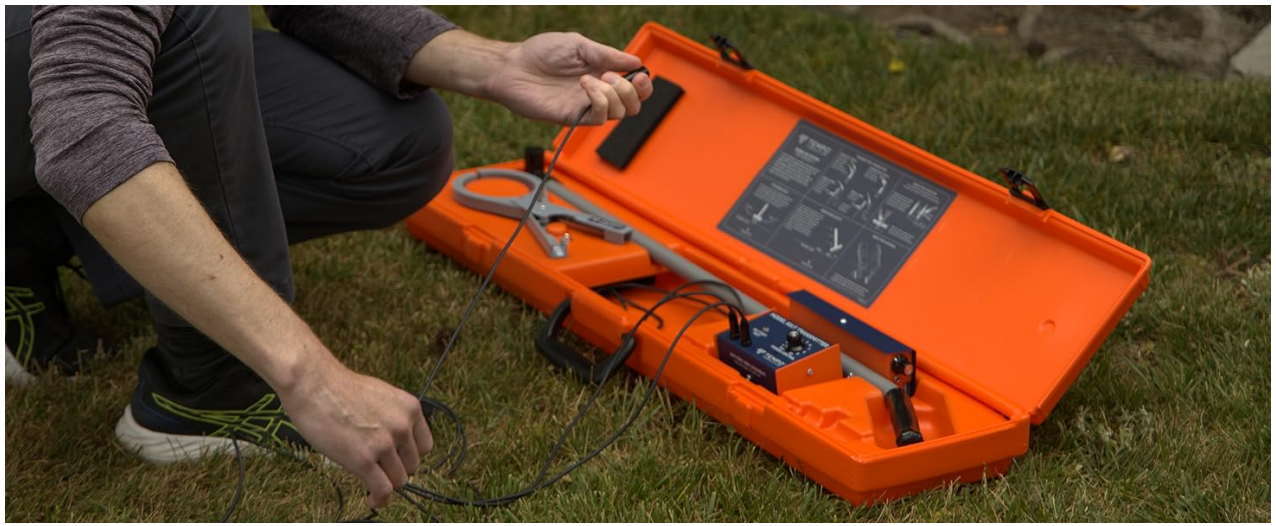
Figure 5: A user demonstrating the use of the A-frame receiver to pinpoint an underground fault.
