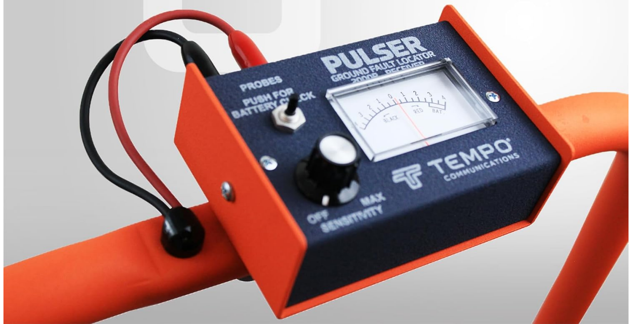
Figure 2: Close-up view of the PE2003-G A-Frame Receiver, showing the meter and controls.
