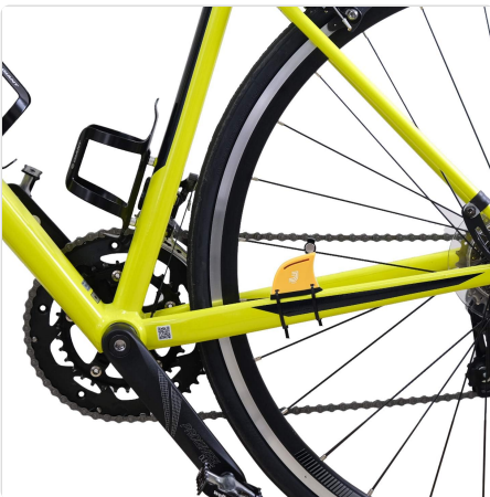
Figure 3: Sensor installation on a road bike with a trainer stand.
