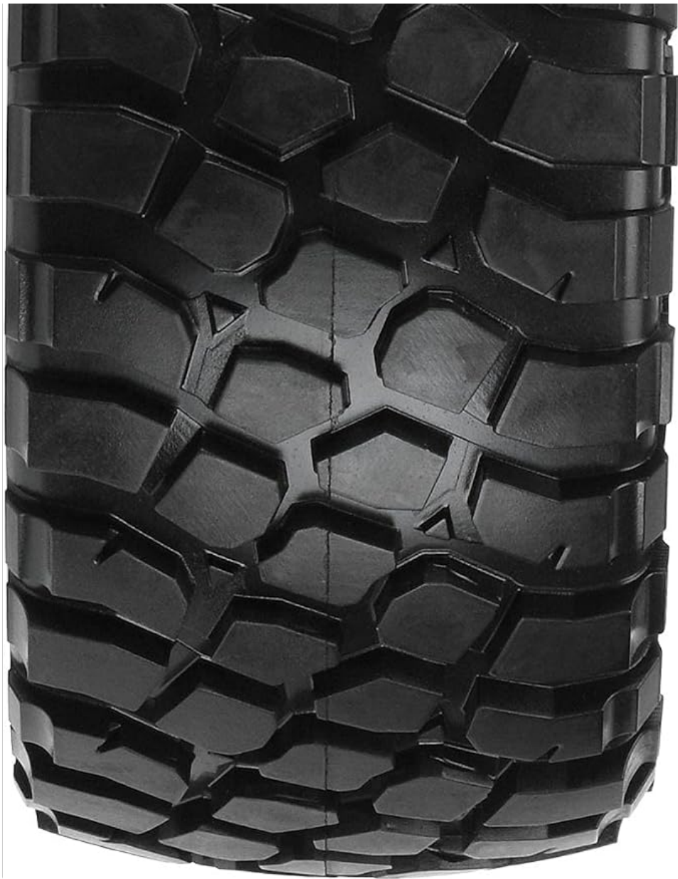
Image 5.2: A detailed view of the tire's tread pattern, highlighting the block design for optimal grip.
