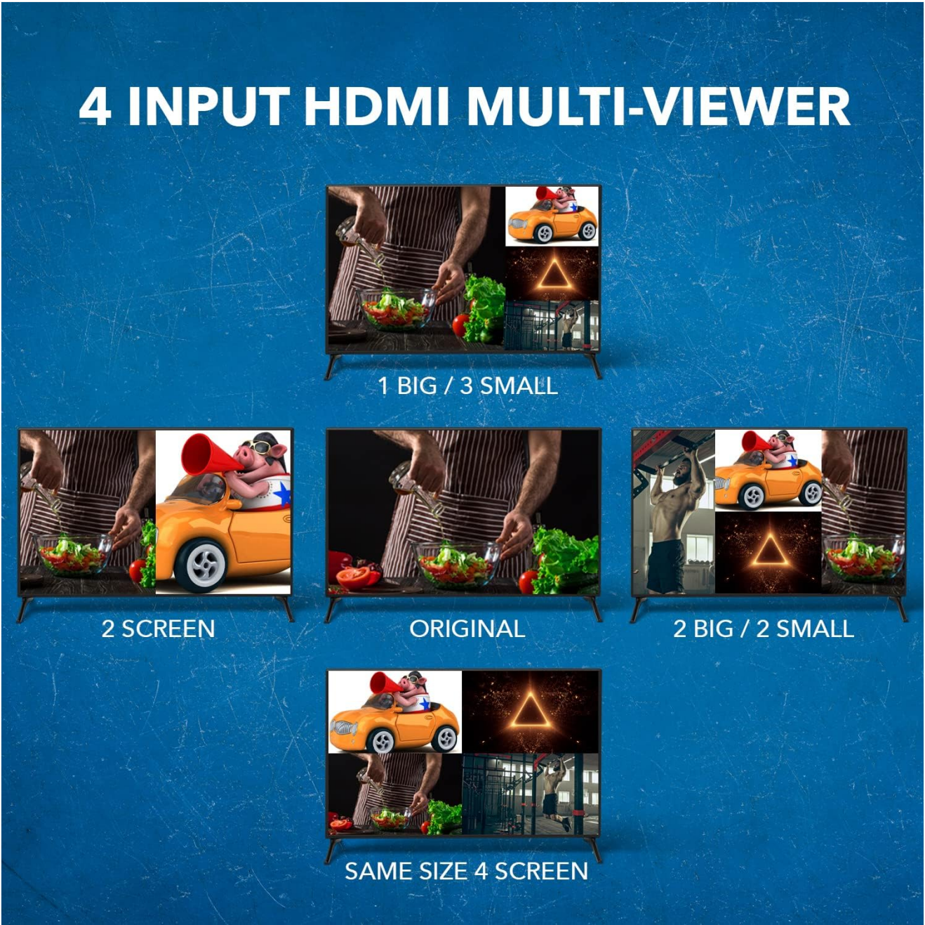
Image: Visual representation of the five available display modes, including 1 Big / 3 Small, 2 Screen, Original (Full Screen), 2 Big / 2 Small, and Same Size 4 Screen.
