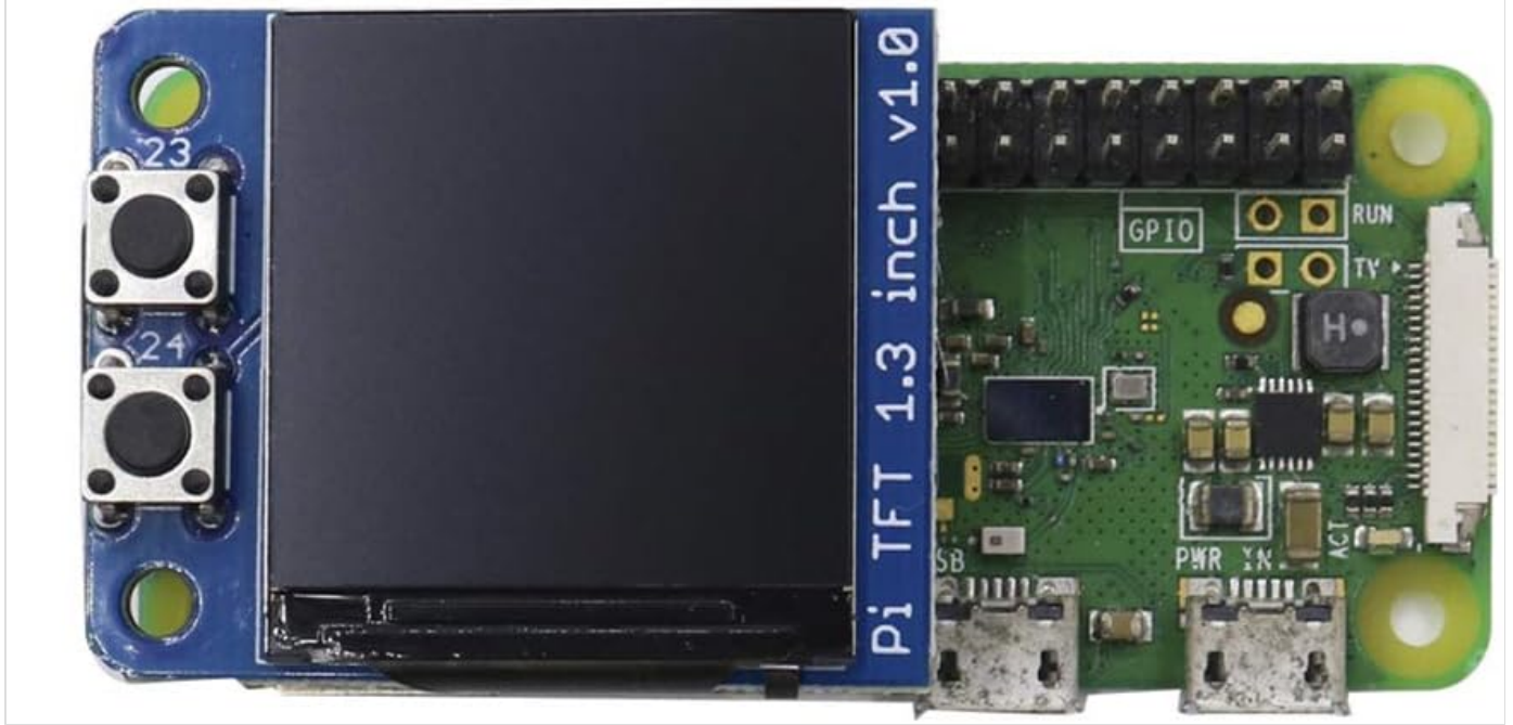
Image: The Mini PiTFT 1.3-inch LCD Display shown connected to a Raspberry Pi Zero, demonstrating its compact size and integration.
