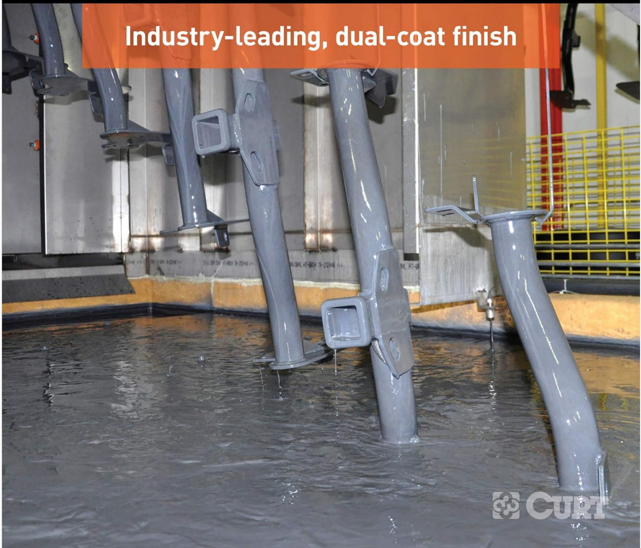
Figure 5.1: Dual-Coat Finish Application Process
