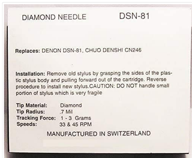
Packaging reverse side displaying installation instructions and technical specifications for the DSN-81 replacement needle.
