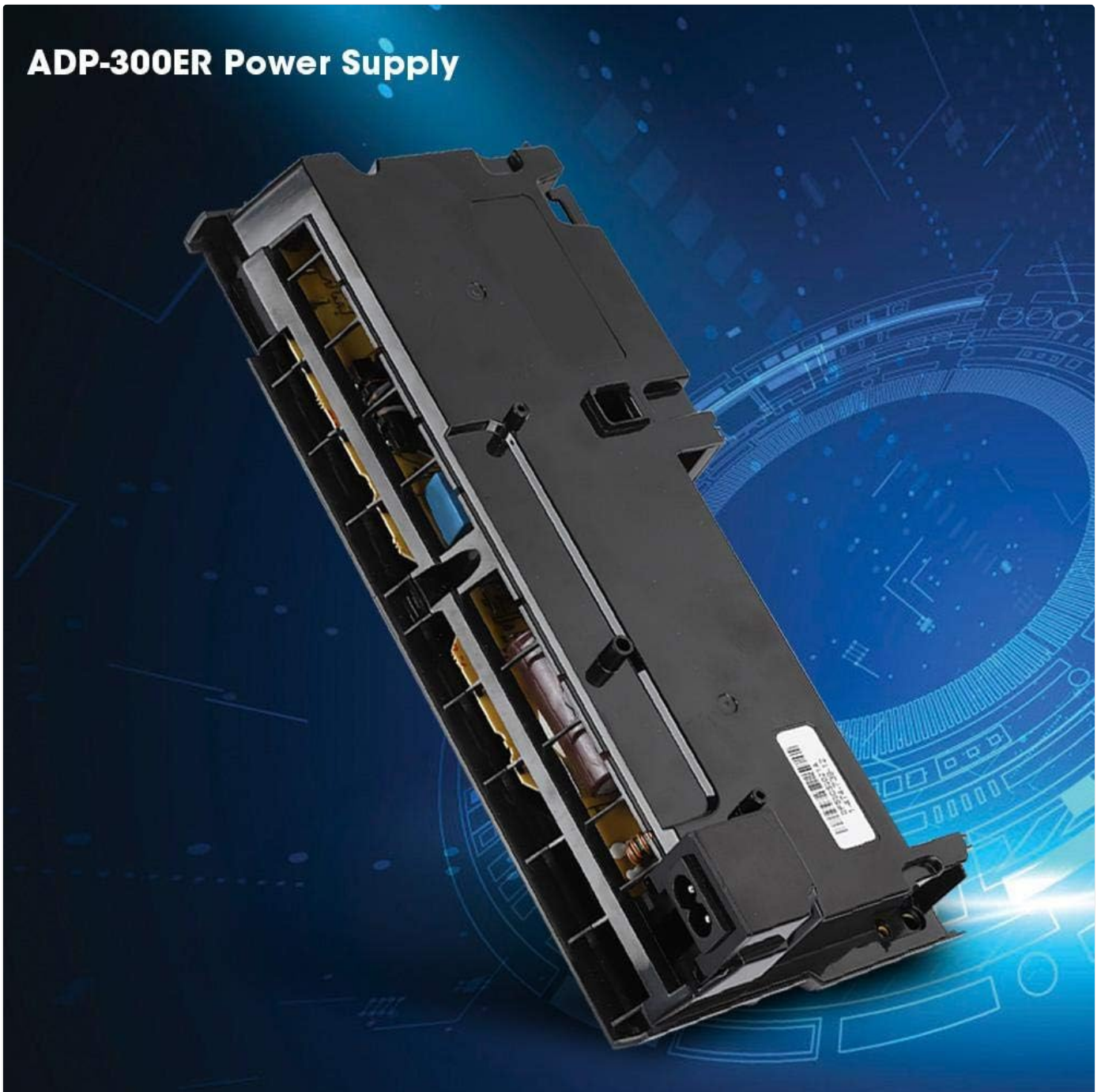
Image 8.1: The power supply unit, showing its model designation, confirming it is the ADP-300FR (sometimes labeled as ADP-300ER) power supply for the PS4 Pro.
