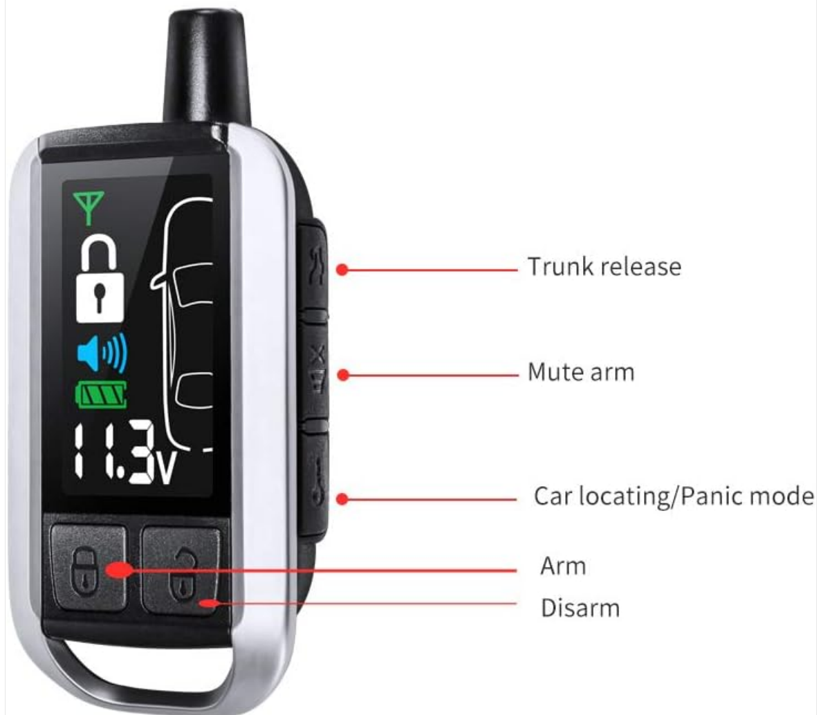
Figure 2: Remote control button functions. The side buttons are for Trunk Release and Mute Arm. The front buttons are for Arm, Disarm, and Car Locating/Panic Mode.
