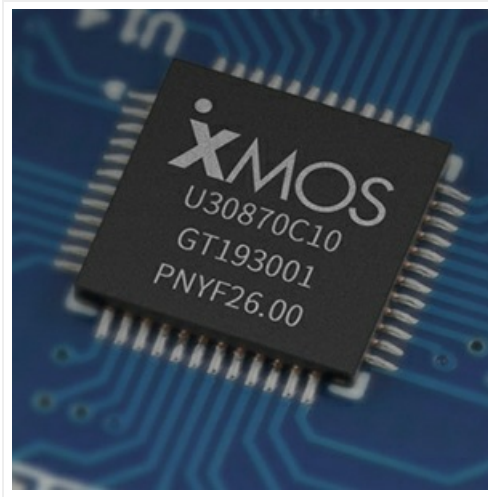
Image: A close-up view of the XMOS XU208 chip, central to the DAC's USB interface.
