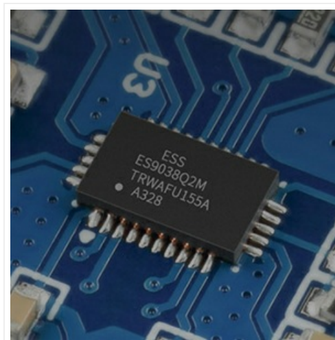
Image: A close-up view of the ESS ES9038Q2M HIFI DAC chip on the circuit board.
