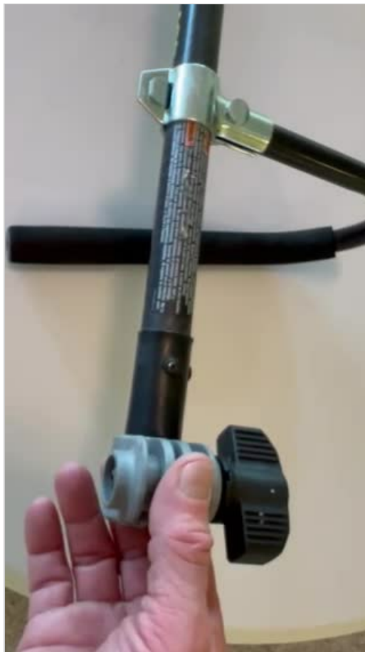
Figure 5: Example of a damaged attachment shaft, requiring replacement.
