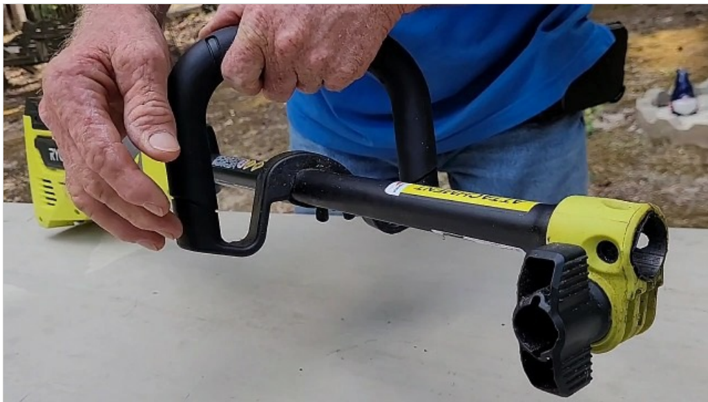
Figure 3: The quick-attachment mechanism for Expand-It accessories.
