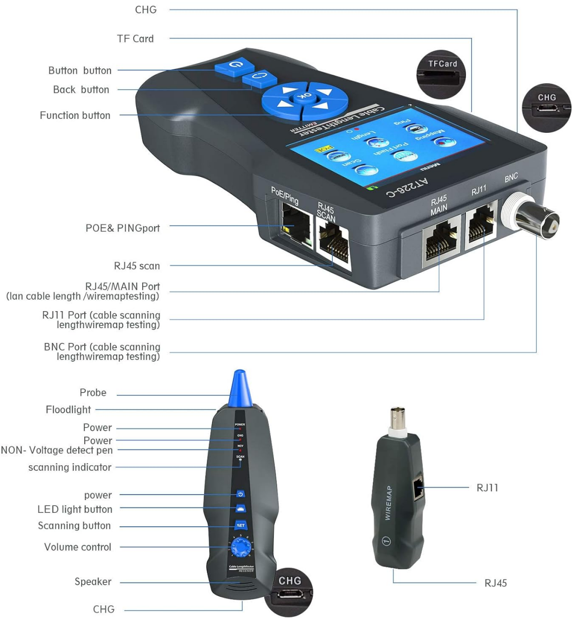
Image 3.1: Detailed view of the AT278 main unit ports and features.
