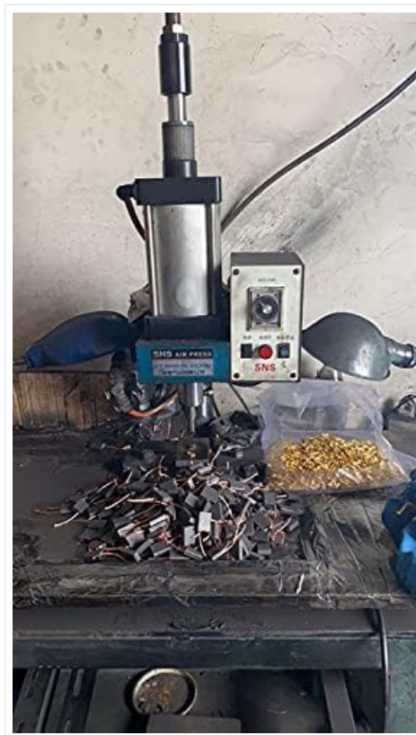
Image: An industrial machine in operation, showing the manufacturing process of carbon brushes. This highlights the precision involved in producing these components.
