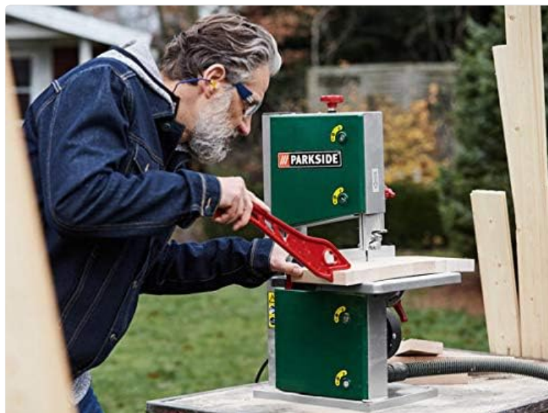
Figure 5.1: Proper operation of the band saw with a push stick.
