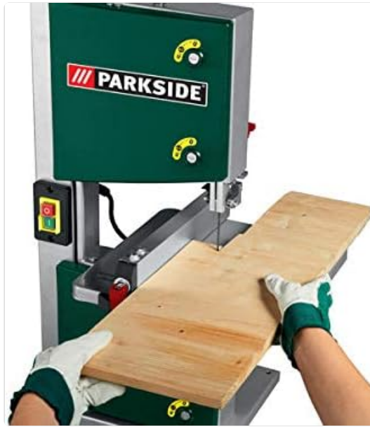
Figure 5.2: Guiding a workpiece through the band saw.
