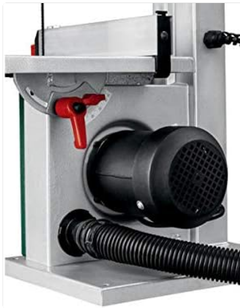
Figure 6.1: Dust extraction port on the band saw.
