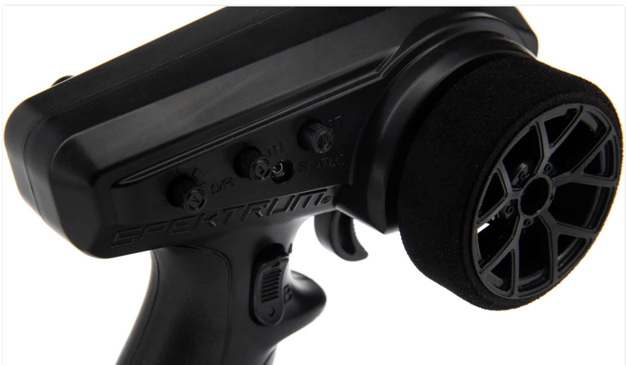
Image: Close-up of the A/B rocker switch, positioned for thumb access on the side of the transmitter.
