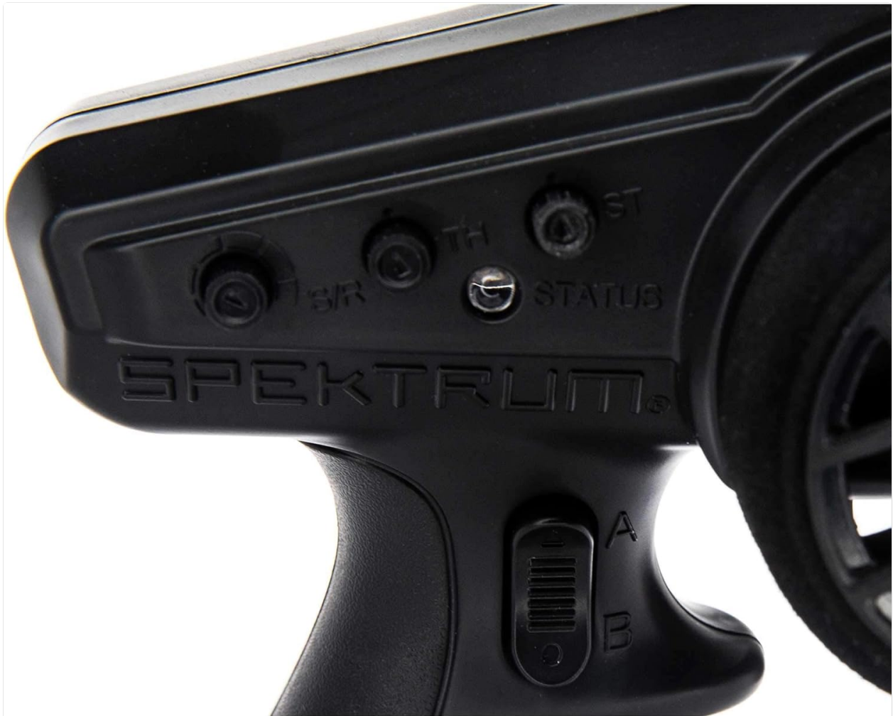
Image: Close-up of the A/B rocker switch, positioned for thumb access on the side of the transmitter.
