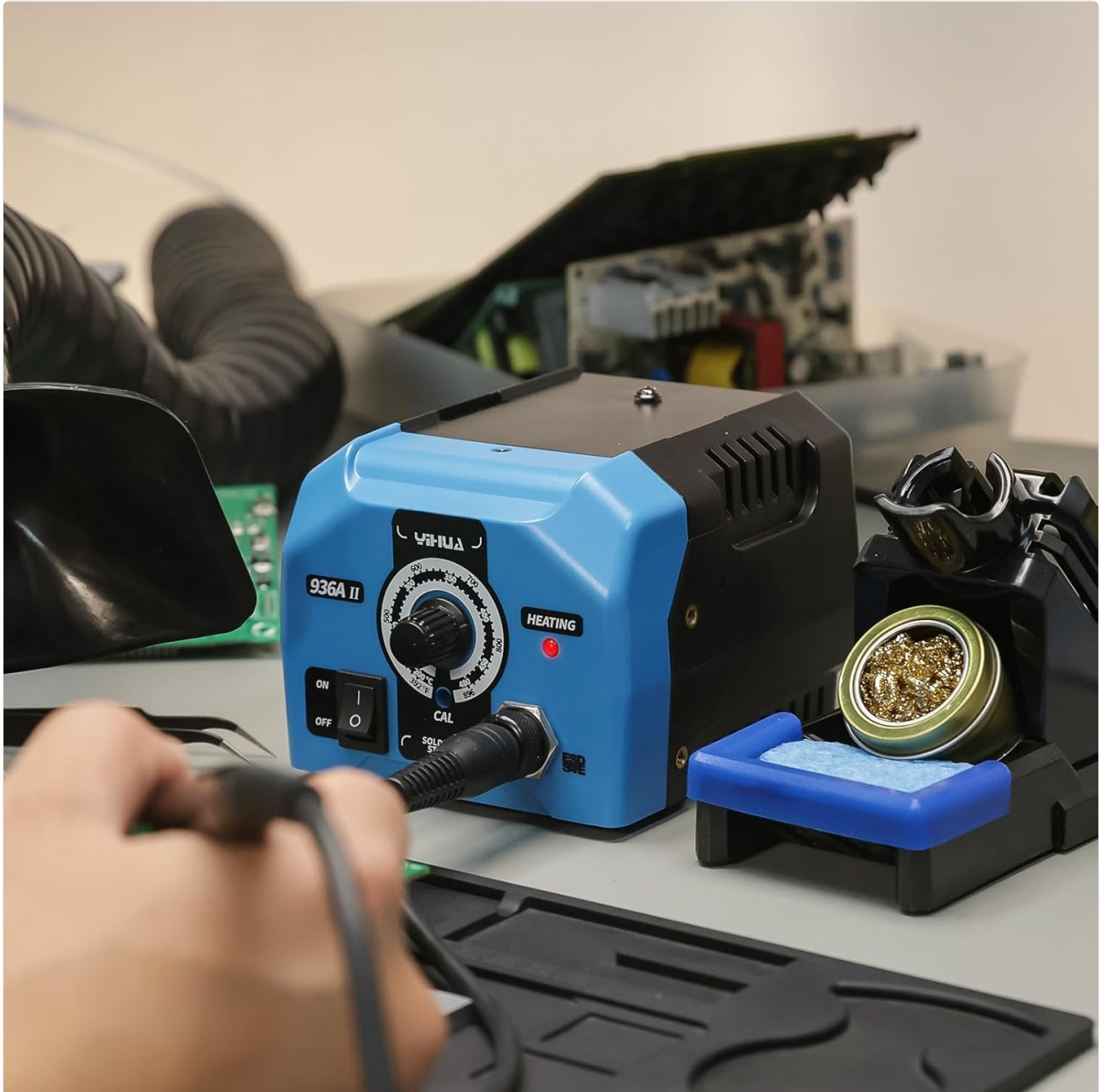
Figure 5.1: Visual guide for initial setup and operation. Steps include connecting the iron, turning on the unit, coating the tip with solder, observing the indicator light, cleaning and tinning the tip, and safely storing the iron after use.
