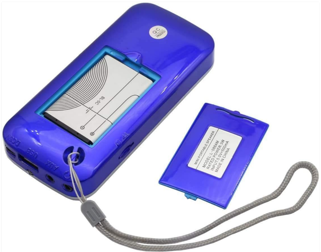
Figure 2: Proper insertion of the BL-5C battery into a compatible portable speaker. Ensure correct alignment of terminals.
