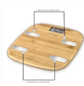
Image: A detailed view of the scale's surface, highlighting the four metal electrodes essential for bio-impedance analysis. Users must stand barefoot on these electrodes for accurate body composition measurements.
