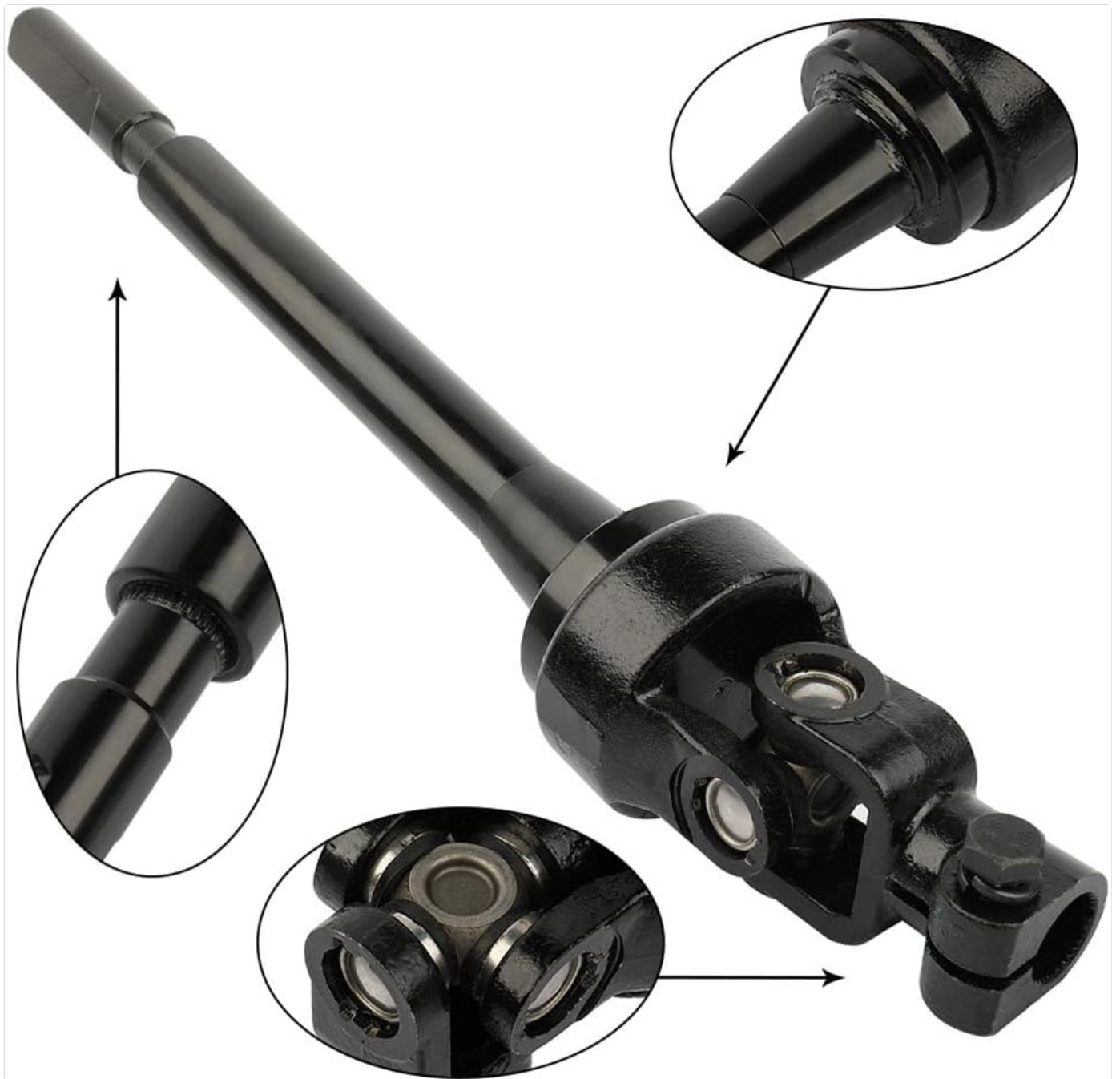
Figure 2.2: This image highlights the universal U-joint coupler and the spline end of the steering shaft, showing key connection points.
