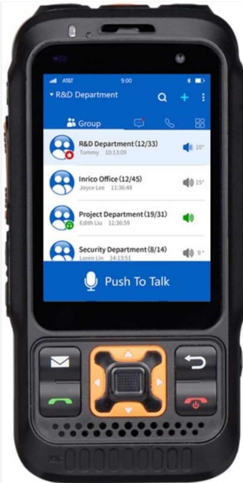
Figure 1.1: Inrico S100 4G POC Radio
