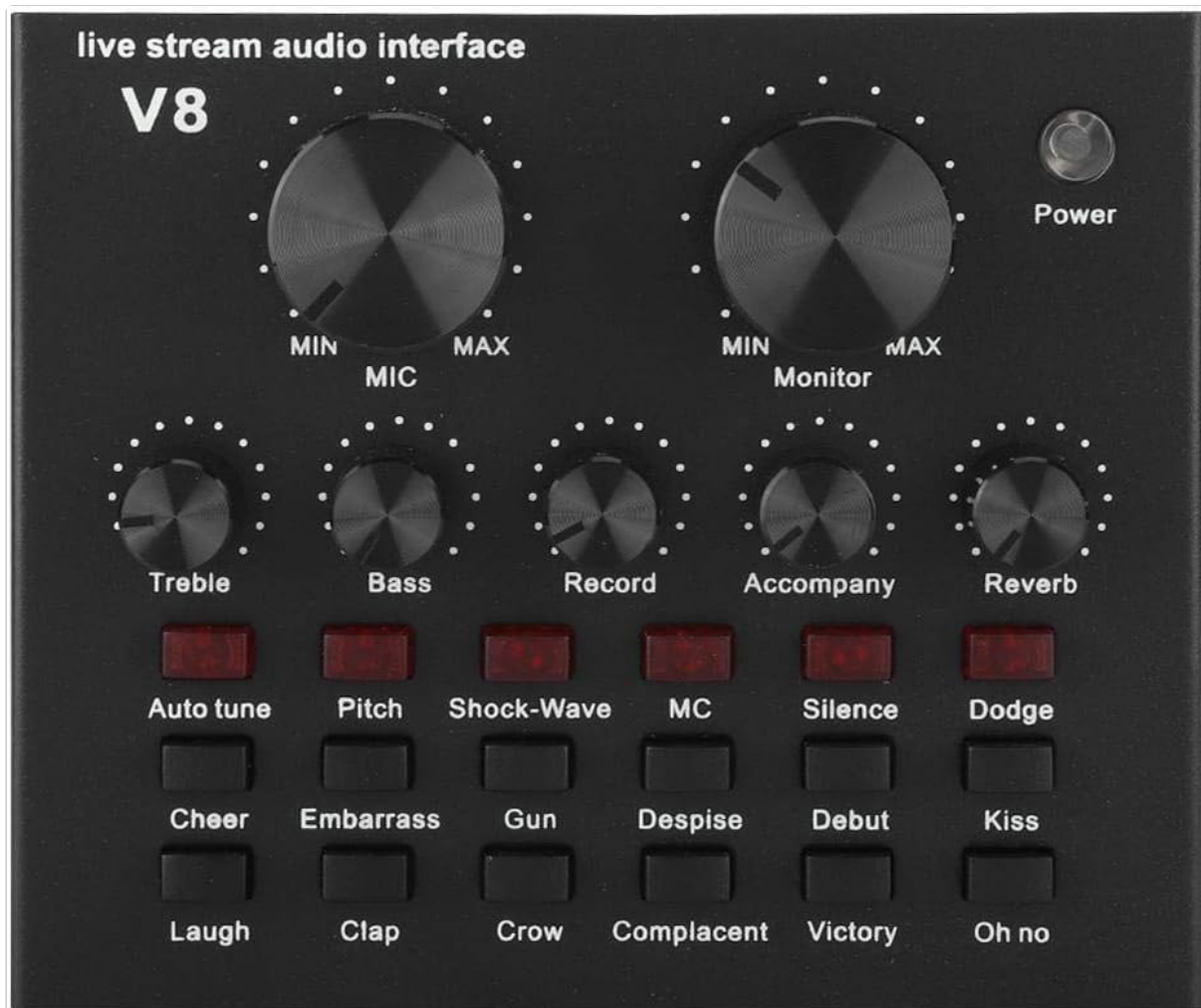
Figure 4: Front panel layout of the V8 Sound Card.
