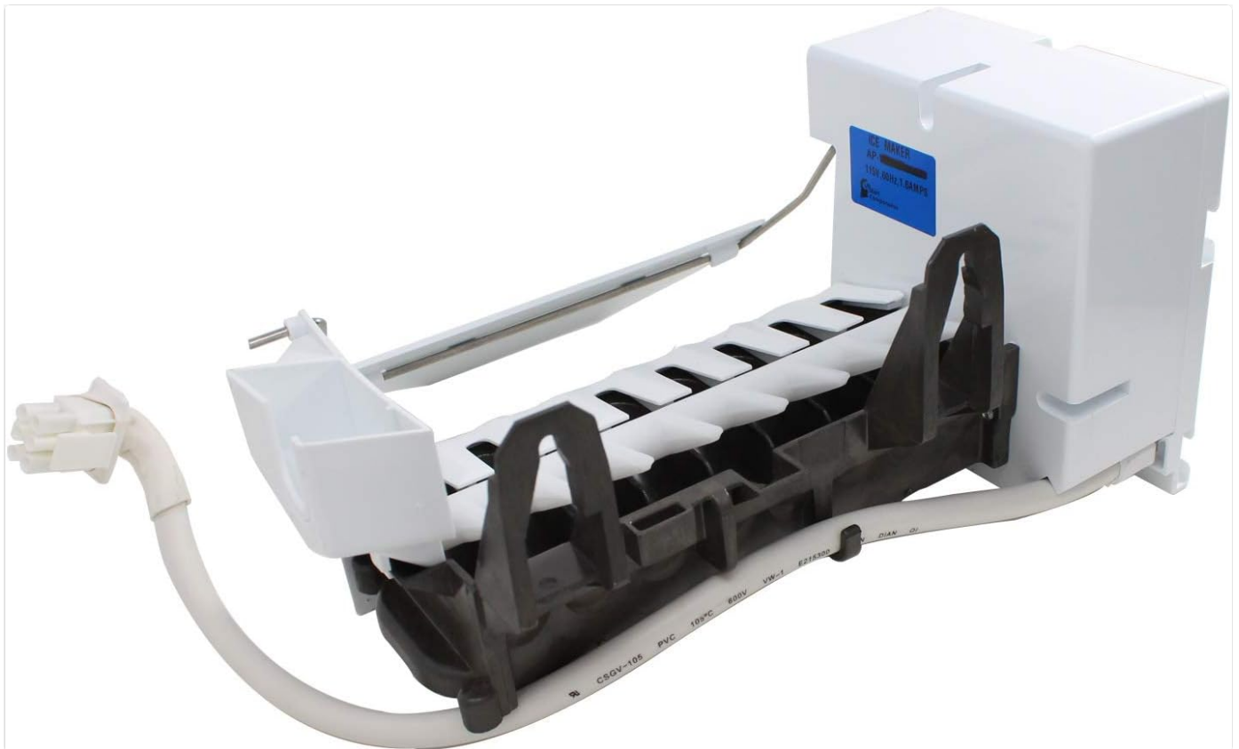
Figure 2: Side view of the ice maker showing the shut-off arm. This arm detects the ice level in the bin and stops ice production when the bin is full.
