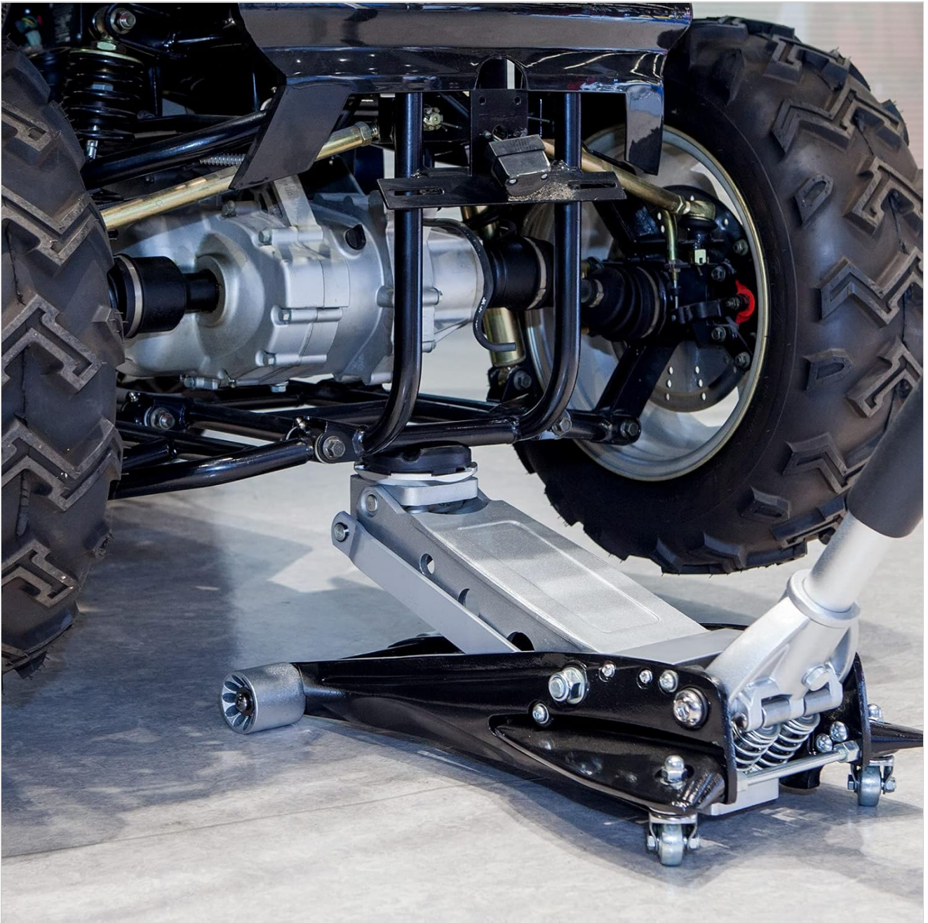
Image: A hydraulic jack with the BIG RED AT83502T-3AB jack pad lifting a vehicle, demonstrating proper application.
