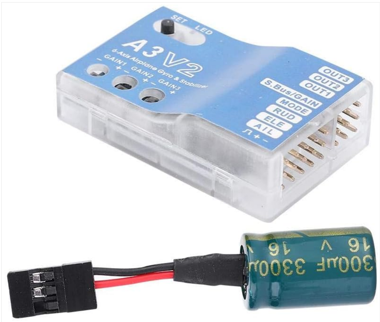
Figure 5.2: Detailed view of the Factory A3 V2 flight controller stabilizer, showing its various input/output ports and gain adjustment potentiometers.
