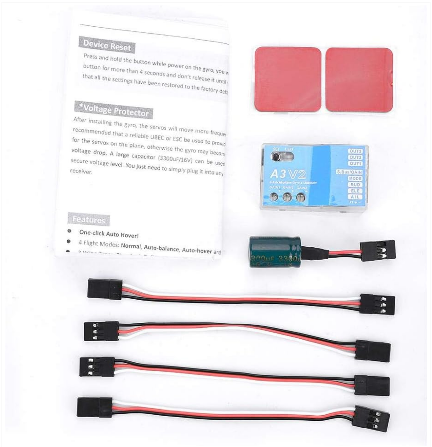
Figure 3.1: Overview of the Factory A3 V2 flight controller stabilizer, including connection cables and capacitor.
