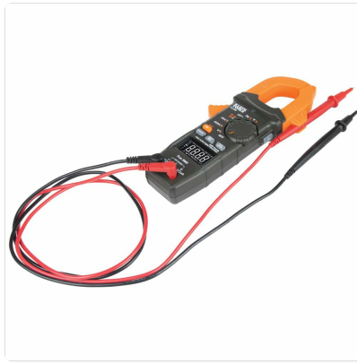
The CL390 with red and black test leads properly connected.
