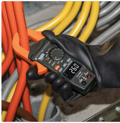
Measuring AC current with the clamp jaw around a single conductor.
