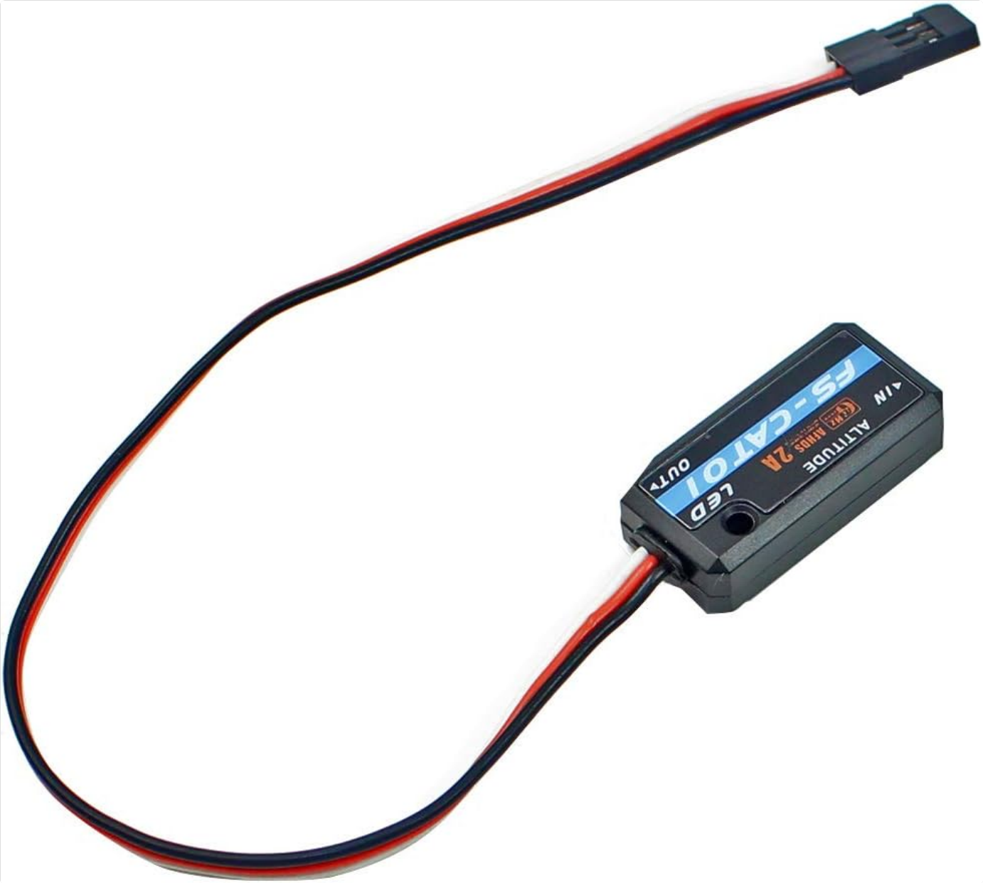
Figure 2.5: The Flysky FS-CAT01 module with a longer three-wire cable, showing the standard servo-style connector for receiver integration.
