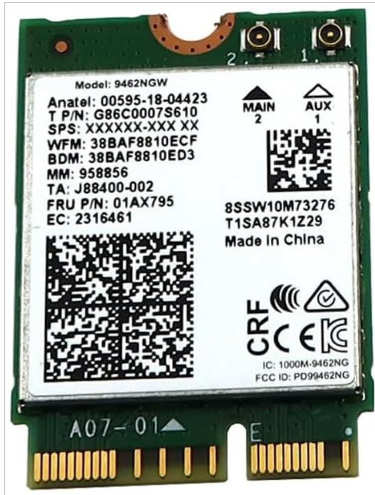
Image showing the Intel 9462NGW M.2 WiFi card with its model number, part numbers, and antenna connectors clearly visible. Note the "MAIN" and "AUX" labels for antenna connection.
