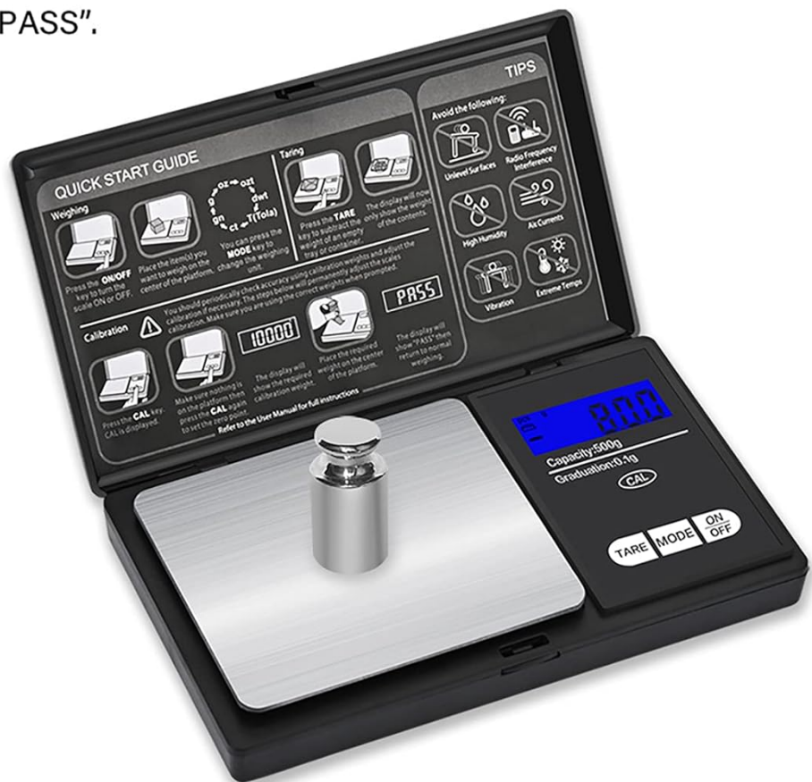
Figure 4: Visual guide for the calibration process, showing the scale with a 100g calibration weight.
