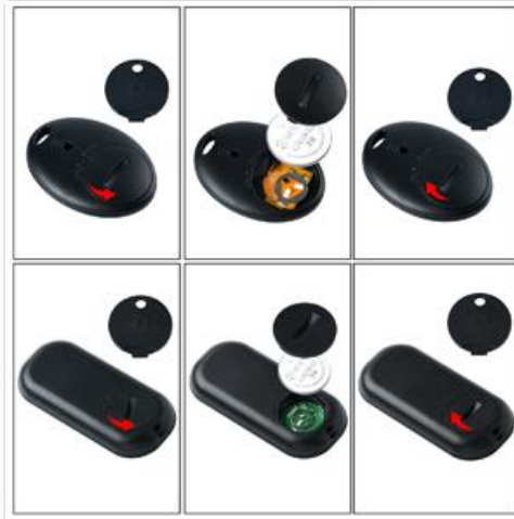
Image: Visual instructions for opening the battery compartment and inserting CR2032 batteries into the devices.
