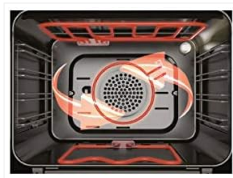
Figure 5.1: Illustration of the convection fan distributing hot air throughout the oven cavity for even cooking.
